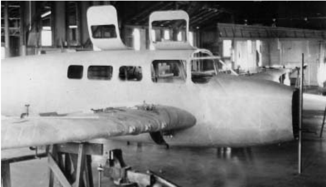
One of an extremely rare group of photographs depicting the incomplete Executive being built in the Big Barn on the Bowlus Ranch at San Fernando, California. The image was probably exposed in early 1936. Discernable in this view is the 45 degree lay up of the grain of the plywood. Each layer would have been applied directionally opposite to the previous one.
