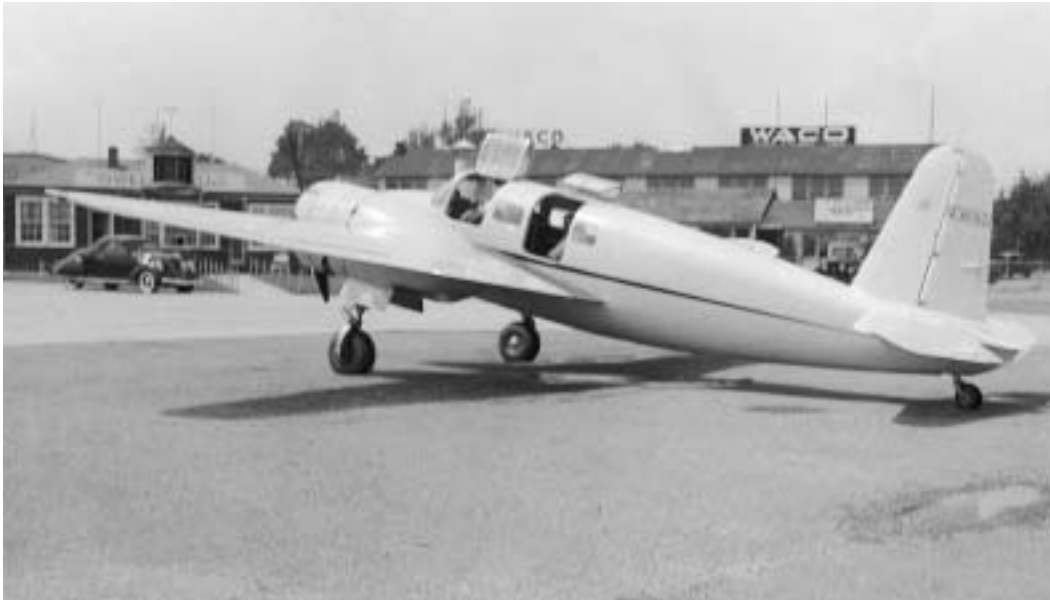
The BTC-1 showing the cabin and cockpit doors in the open position. The centerfold device of the doors is evident.
