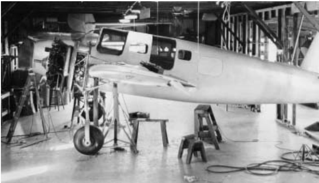
The Bennett further along in the assembly process at the Bowlus Ranch. The engines and landing gear had been installed in the nacelles.
